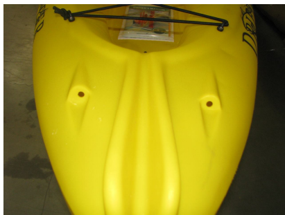
Fig.#C Stern Cable Holes
